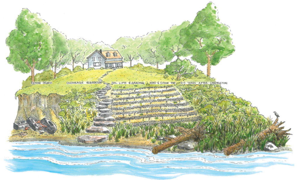
A concept drawing of channel bank treatment options.
